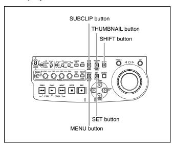
With the THUMBNAIL button off, hold down the SHIFT button and press the SUBCLIP button.
